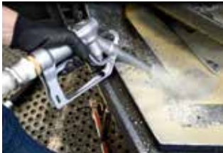
Flux inversion liquids discharge system ( 26 gal/min)
