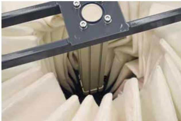
AUT: Automatic filter cleaning system
