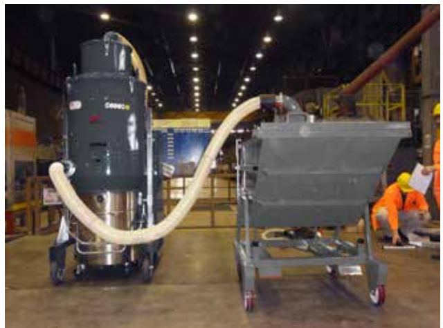
Tilting pre-separators, high capacity (106 - 158 gallons)
